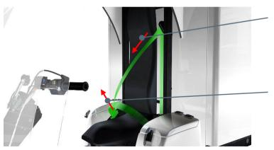
Retractor test: rapidly and strongly pull,
