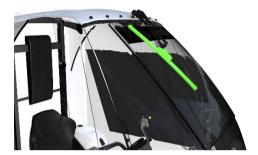
• Pull the wiper blade out of the arm-attachment (to the rear and upwards)
