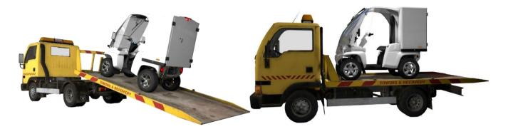
Secure the Paxster on the platform like all cars by clamping / strapping the wheels down to the platform.
