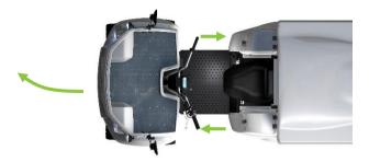
Keep both hand on the grips of the steering bar. If possible, use the throttle to move the vehicle some centimeters while steering.
