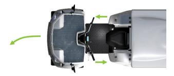
Keep both hand on the grips of the steering bar. If possible, use the throttle to move the vehicle some centimeters while steering.
