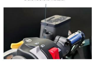
To refill DOT4 brake fluid, unscrew the top-lock and temporarily remove the rubber sealing.
