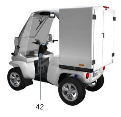
Unscrew the star-lock screw manually and open the hatch to access the fuses.
