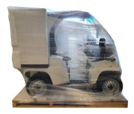
Ensure the vehicle is tied down to the pallet on all 4 wheels.
